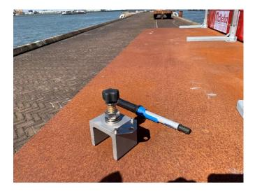
The testing tool can check the holding force of the magnet.
