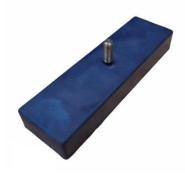
RMB, Rubber Magnet Blok Dimensions 201x61x 28 mm. Magnetic force : circa 400 kgf on untreated steel Tested pullingforce: 350 kgf op 0,2 mm paintlayer and 12 mm steel Tested shearforce : 250 kg op 0,2 mm paintlayer and 12 mm steel Magnetmaterial : Neodymium, Studbolt : M10x26 Material studbolt : Stainless Steel WS. 1.4404 Rubber coating : EPDM
